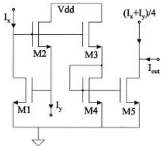
Fig. 4. Geometric mean circuit—a “stacked MTL” implementation.
