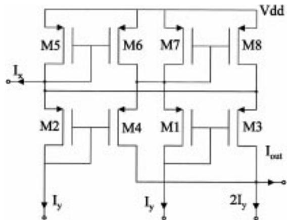
Fig. 6. Current squarer/divider—an “up-down MTL” topology.
