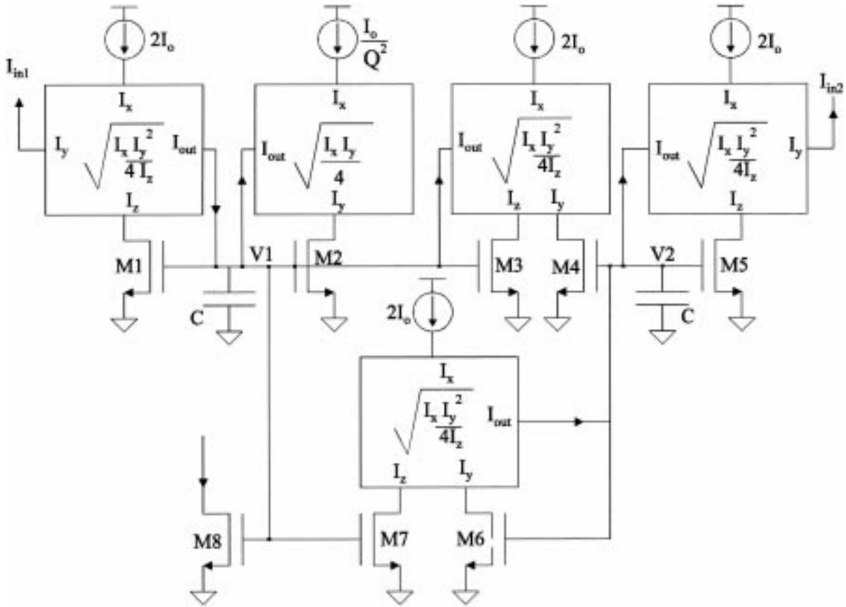
Fig. 3. A block diagram implementation of a square root domain biquad filter.
