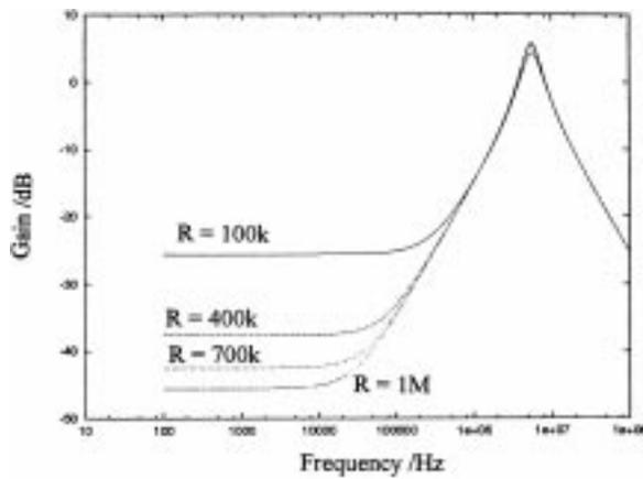
Fig. 8. Simulation results of a behavioral model of the biquad filter, demonstrating the degradation in stopband attenuation with decreasing sub-circuit output resistance.
