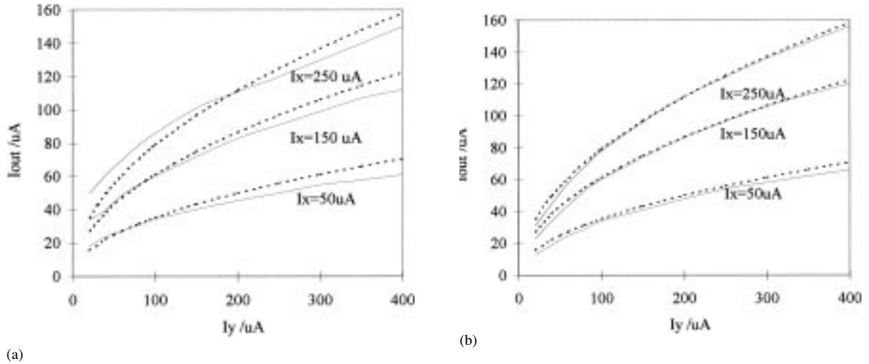
Fig. 5. Comparison of ideal and simulated results for the “stacked MTL” geometric mean with (a) body effect included and (b) no body effect.
