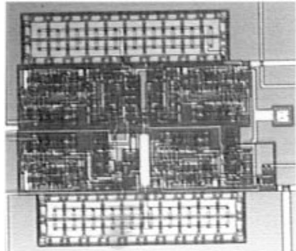
Fig. 9. Microphotograph of the biquad filter.
