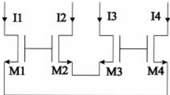
Fig. 2. A four-transistor NMOS translinear loop.
