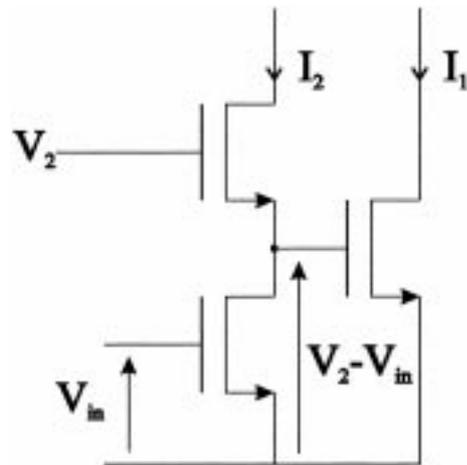
Fig. 1. Linear transconductor based on the MOSFET square law characteristic.
