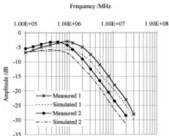
Fig. 10. Comparison of simulated and measured biquad bandpass response.
