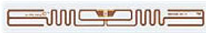
Figure 1.4: A typical UHF RFID tag with meandered dipole antenna
